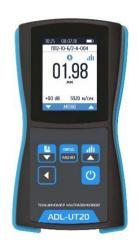
Ultrasonic thickness gauge ADL-UT20 can work with any separately combined transducers operating at frequencies from 2.5 MHz to 10 MHz, their use provides high reliability of results in laboratory, workshop and field conditions.
